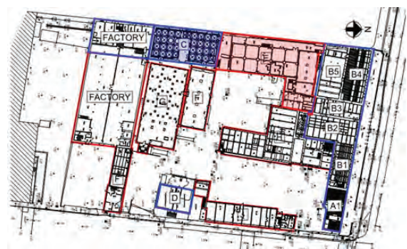
Plan view of site in 2013. Buildings outlined in blue were retained and those in red were demolished. The two buildings referred to in the example (Buildings C and E) have been shaded. © Arup
