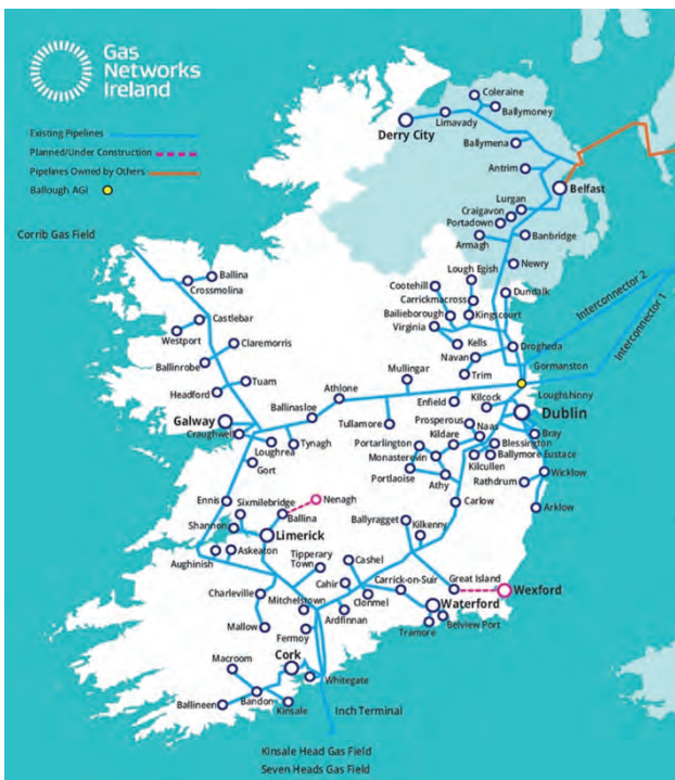
Irish Gas transmission network
